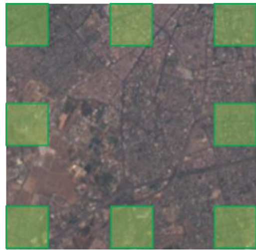
Figure 11. Image edge inspection using mosaic padding
